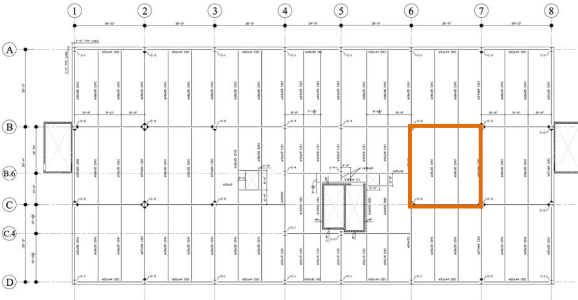
Figure 1.1 Typical Floor Framing System
